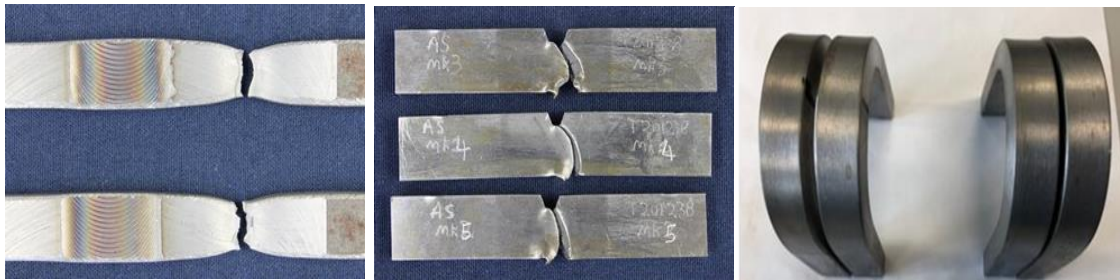
Figure 3. Tensile, Charpy impact and bend test samples of friction stir welded steel.
