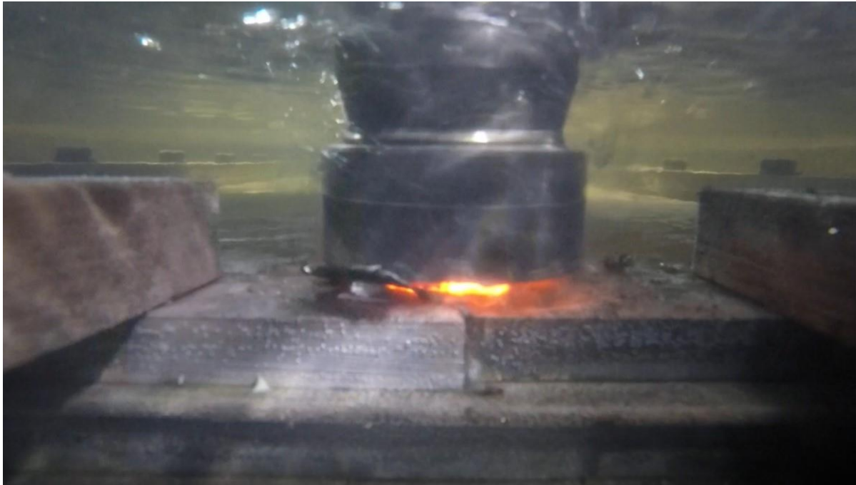
Figure 6. A friction stir butt weld being made under water to join two 12mm thick steel plates.
