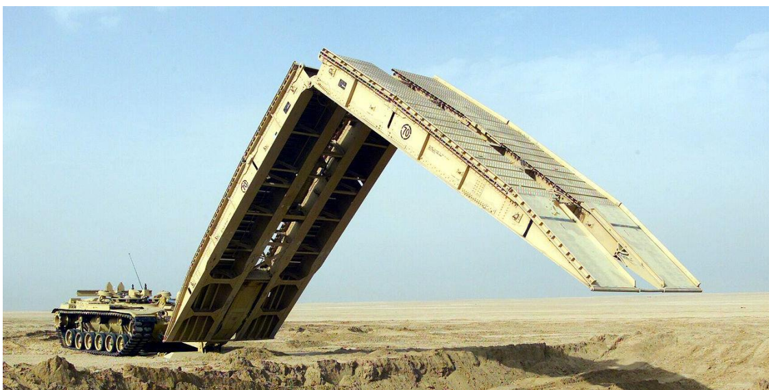
Figure 17. Dry gap crossing with an Armoured Vehicle Launched Bridge (AVLB) (US Army)
