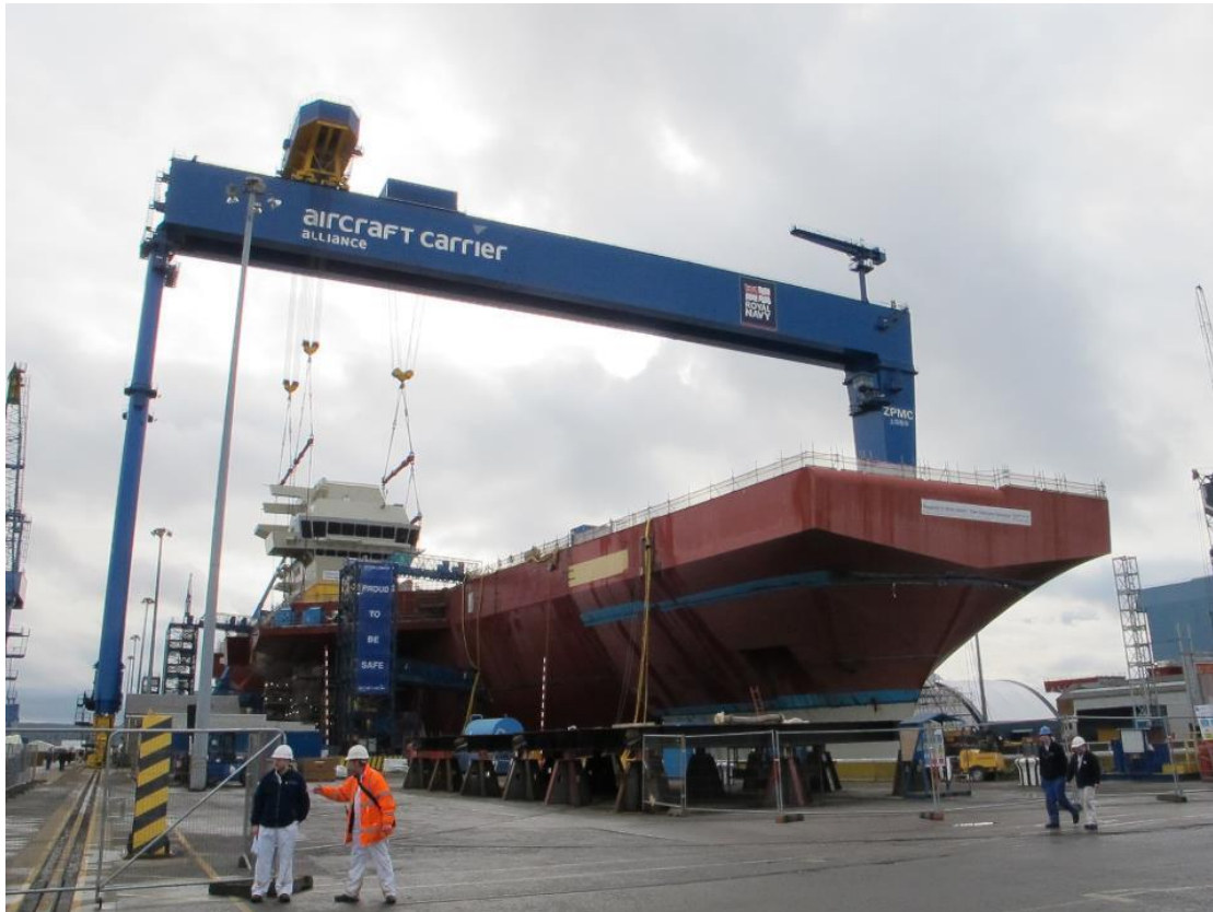
Figure 19. Gantry and portal cranes could benefit from FSW, having potentially greater spans and / or lifting capacity.
