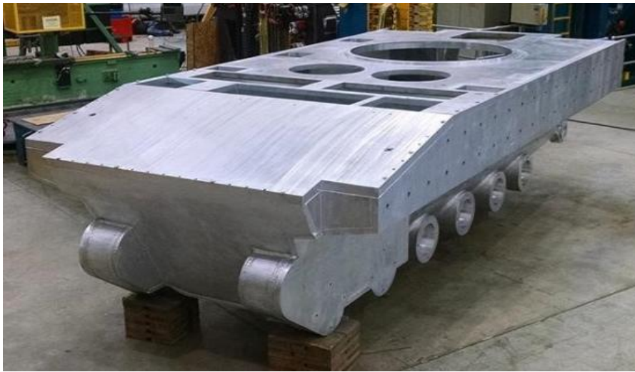
Figure 16. Friction stir welded AFV hull in aluminium. (Concurrent Technologies Corp)
